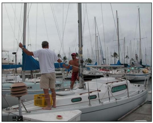
tem can be used to lower the mast to pass under bridges as the mast can be left in the down position while the boat is under power in calm water. For variations and more ideas on the bridle system, see:
