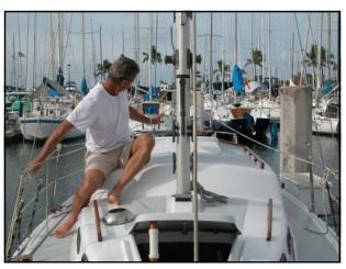
Square up the boom and snug up the bridle so the boom is centered and at right angles to the mast. The weight of the mast will be supported by the halyard and the tackle. The bridle will keep the boom centered and prevent it from flopping to one side as you lower away while keeping tension on the upper shrouds.
