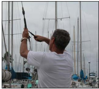
Now you can disconnect the after lower shrouds and back stay. First disconnect the backstay and take it to the mast. If you don't have a helper, tape it or tie it. Then bring the after lower shrouds to the mast and secure them. The forward lowers and the forestay do not need to be disconnected. The upper shrouds are attached to the bridles
