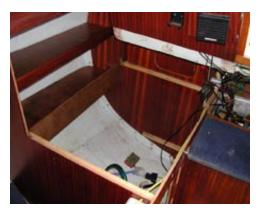
space for the wooden base, supporting the fridge (See Item 7). Dimensions given are outer-dimensions of the box with a 2mm margin for finishing. The volume is minus 50mm foam thickness on all sides. Make a template of the box where the insulation sheet for
