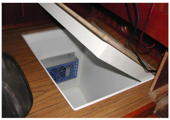
A personal choice. You may choose for example a Danfos compressor and cooling armature like your fridge at home. In that case you can install the compressor in the starboard cockpit locker next to the dustbin. Advantage: You can get things frozen and cooled faster.Disadvantage: More noise, less economical on battery power, needs more space
