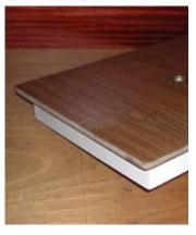
minus 1.5mm margin and 1mm thickness of the edging per side. Sides to be sanded with an electric sander.
