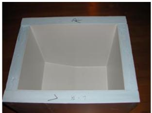
4. To make the construction fit the Vega's shape and to maximize volume (appr. 10 litres) the PVC base sheet should be warmed at the correct place (use a Fan-heater or hot-air paintstripper) and bend to the correct angle along a sharp (table) edge.
